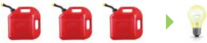
Fuel Used by Power Plant ▶ 290 W Fuel for 100 W
